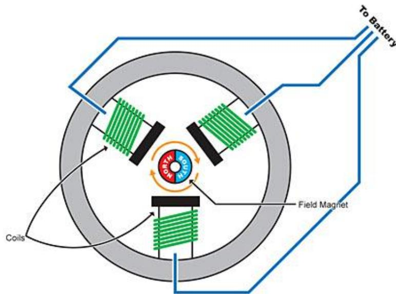
In a brushless motor the permanent magnets are on the rotor (red and blue on diagram), and the windings of wire (green in diagram) are on the can - or stator. Different amounts of current are supplied through three wires (blue in diagram). Basically one wire supplies positive current, one negative, and the third is ground at any given time. This makes two of the windings of wire into electro-magnets that attract or repulse the permanent magnets in the rotor which spins as a result.
